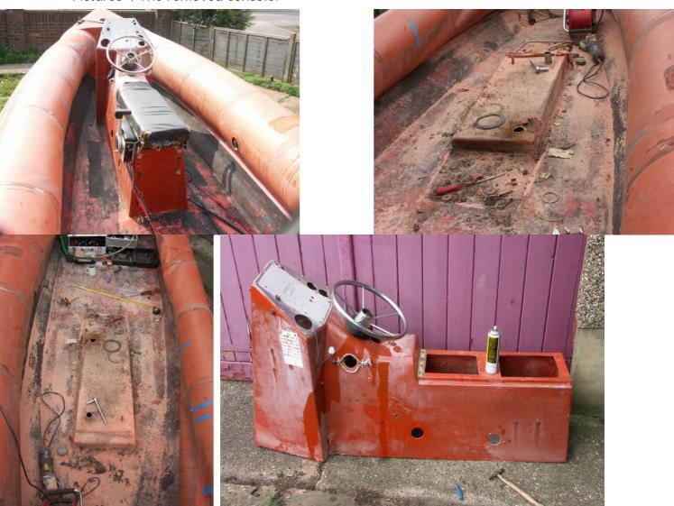
Having removed the console it was time to look at the semi-under deck fuel tank, the current position of the tank is to far forward and would stick out of the front of the new console, so I have
